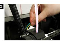
Remove the motor wire harness connector from the port at the top of the extruder motor.
