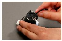
Use the 2 mm hex wrench to remove the two bolts holding the drive block to the motor.
