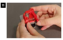
Orient the bearing arm so that the bearing is at the left and the bearing cover faces up. Then line up the corresponding bump on the bearing arm with the other end of the spring.
