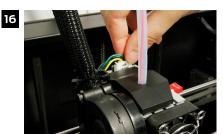
Return the motor wire harness connector to the port at the top of the motor.
