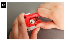
Pinch the front side of the drive block base and the long side of the bearing arm together to compress the spring. Compress the spring until the bolt hole in the bearing arm and the remaining bolt hole in the drive block base line up.
