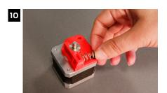
Fit one end of the spring over the round bump on the drive block base. The bump protrudes horizontally from the lower right corner of the drive block base.
