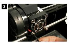
Use the 2.5 mm hex wrench to loosen the two bolts at the lower corners of the front extruder fan.
