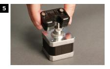
Remove the drive block. You can put the drive block and bolts aside. You will not need any of these parts to complete this part replacement.
