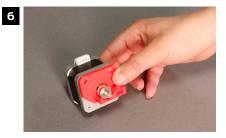
Add the new drive block base to the motor so that the flat side rests against the top of the motor, the large hole at the center fits over the drive gear, and the two bolt holes in the base line up with the bolt holes farthest from you on the motor.
