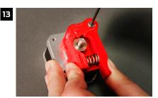
Push the shoulder bolt through the bolt hole at the corner of the bearing arm and the drive block base and into the bolt hole on the motor. Make sure the holes on the bearing arm and motor are perfectly aligned before inserting the shoulder bolt.
