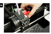
The new drive block is now fully assembled. Return the motor assembly to the extruder. Slide the motor assembly back into the extruder.
