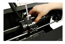
Set the motor assembly down on a work surface. Orient it so that the motor shaft points up and the motor wire harness connector is on the side farthest from you.
