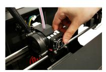
Pull the bolts, fan guard, fan, spacers and heatsink about half an inch out of the extruder as one piece. This will freethe motor. Do not pull the screws out all the way. Pull the motor assembly out of the extruder.
