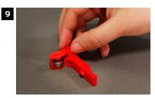
Add the bearing cover to the bearing arm so that the flat side faces up, the more rounded end fits into the round depression at the corner of the bearing arm, and the less rounded end partially covers the bearing. Press the cover on until it is flush with the edges of the bearing arm.
