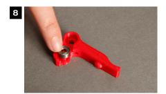
Set the bearing arm down on your work surface with the flattest side facing down. The bearing arm is roughly L-shaped, and on the short side of the L you will see a short post pointing upward. Add the radial bearing to this post.
